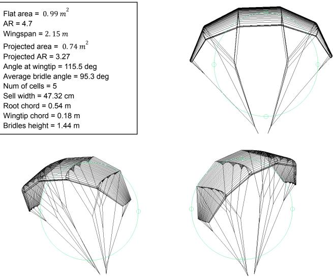
The reason we choose this type of parachute is to allow us to navigate the CanSat. Our Satellite will have two small arms which will unfold after the release from the rocket and they will steer the glider by breaking down each side of the wing.
