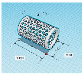
Image 3: Mechanical design of the outer casing
