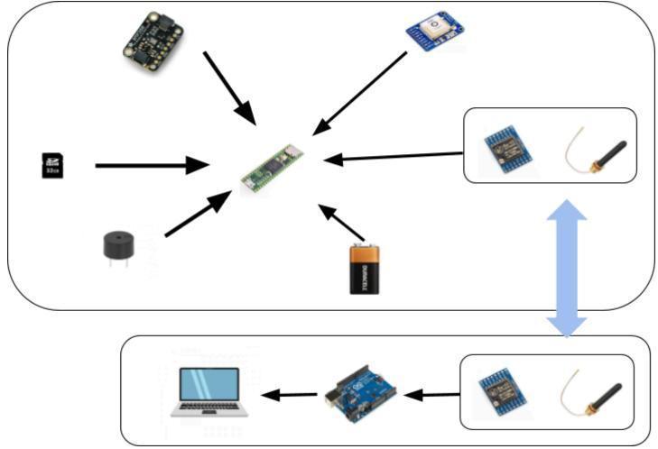
Image 2: Graphic representation of the main components used for the CanSat and Ground Station.
