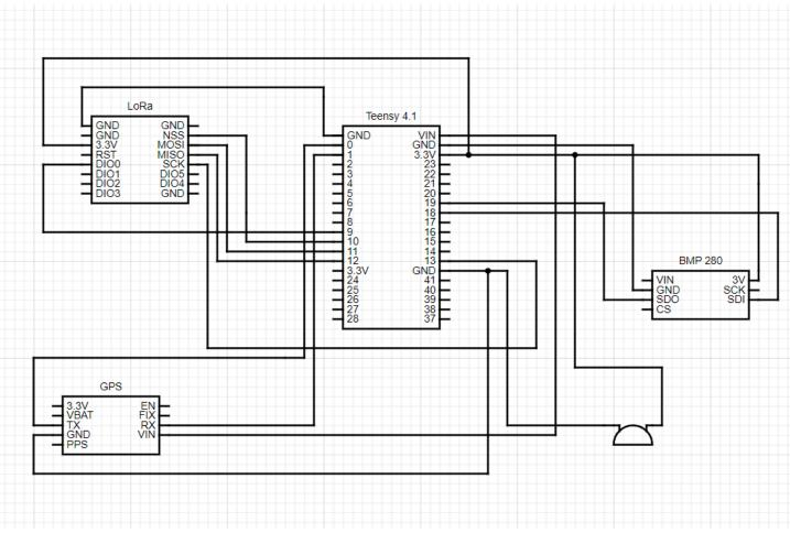
Image 3: Wiring diagram of the CanSat.
