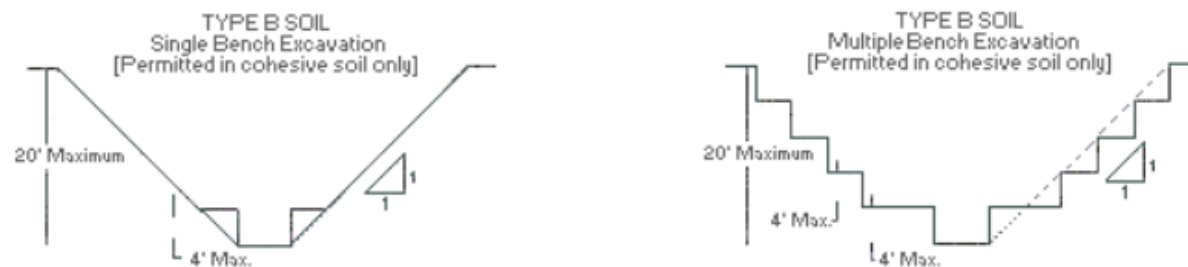
Figure 3: Sloping and Benching Options in Layered Soil
