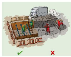
The sides of the excavation or trench should be supported by timbering or other suitable means or sloped and battered back to a safe angle of repose to prevent a collapse. The type of support necessary and angle of repose will depend upon the type of excavation, the nature of the ground and the groundwater conditions.
