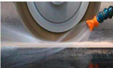
It is also recommended to reduce the rotation speed when the tool enters and exits the slab.
