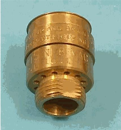
A hose bib *vacuum breaker* is installed on the end of a hose bib (sill cock, boiler drain, etc.) or anywhere a hose can be connected. It contains one spring loaded valve and an atmospheric vent that is controlled by a diaphragm seal. Installation & Use:
