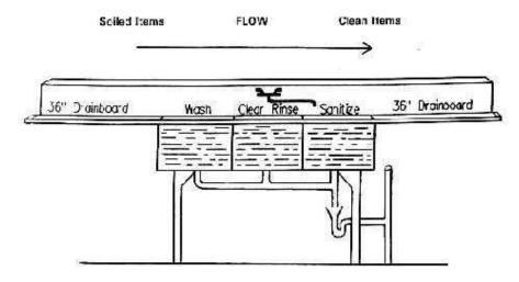
Recommended warewashing arrangement using three-compartment sink. Drainbuards for solled dishes and for cleaned utensits must be adequate. A 36" drainboard should have a pitch of %" to %" per foot toward the sink.
