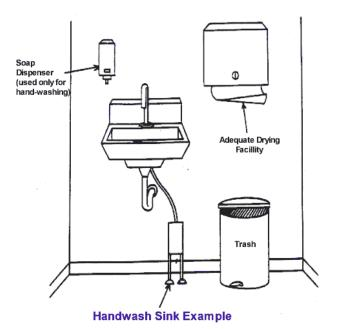
Provide a separate handwashing sink; disposable towels; supply of hand cleaning agent; and waste receptacle for each food preparation area, utensil washing area, and toilet room (required number based on law). Sinks used for food preparation or for washing *equipment* or utensils shall not be used for handwashing.
