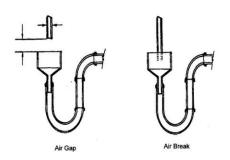
**Air gap:** is the unobstructed vertical space that separates the end of a supply line and the flood rim of a receptacle. The *air gap* must be the greater of either a minimum of one inch or twice the diameter of the supply pipe/
