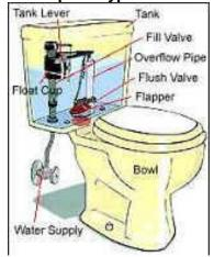
Installation and Use: Ballcock assembly must be installed above the overflow pipe high water level.
