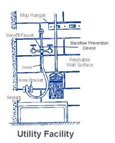
At least one utility sink or curbed cleaning facility with a floor drain shall be provided for cleaning mops or disposal of liquid wastes. The water supply must be protected against backsiphonage (see part 12). A properly sized mop and broom rack shall be provided. All toxic materials including cleaning compounds, pesticides, sanitizers, etc. must be stored in an area away from food preparation.
