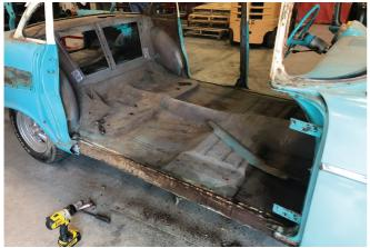
Step 5: Car you're starting with have rusty outer rockers? No worries, they're outta here anyways! The kit put together includes proper 2-door sedan outer rockers, again, all in the name of keeping proportions correct, and being less overall work than trying to section a 4-door rocker.
