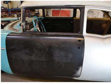
Step 11: Almost there! Here you see everything finish welded and fitted. At this point, you can test fit your mouldings, drill your holes, and make all necessary trim pieces line up exactly how you'd like them.
