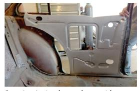
Step 3: A simple mock-up with a section of original-style 2-door inner quarter shows some of the difference in the 2-door and 4-door. Ever seen a 4-door that someone has simply welded up the back doors, and the proportions look off? This is why! The difference shown will be made up by using a proper 2-door sedan front door, and relocating the b-pillar into proper location.
