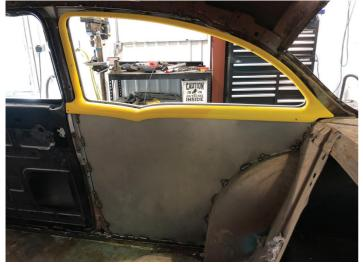
Step 10: With the outside squared away, you can move on to the inside. With the b-pillar and outer quarter in place, you will need to make a few small tabs to attach to the outer quarter to the roof, and provide a way to mount the garnish moldings. The kit from Woody's Hot Rodz comes with 150-style fixed quarter glass and
