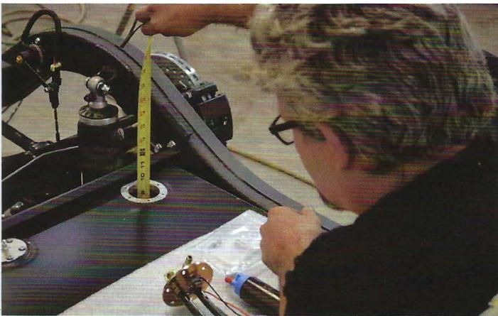
Just like the sending unit, the fuel pump assembly is a universal component that requires roughly the same modifications. Again, make sure these measurements are correct, as incorrect measurements will leave the pickup sock shoved against the bottom of the tank, or too tall to properly utilize
