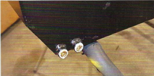
If you're using this tank in a carbureted application, or with an in-line EFI fuel pump, CPP provides you with feeds to do so. We're doing an in-tank setup for longevity and quiet operation, so we plugged these off.
