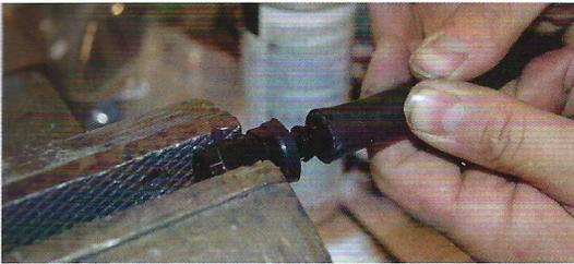
With the filter/regulator mounted, we're onto fuel lines. CPP's fuel kit uses push-lock hose and AN-Style fittings throughout. Assembly is as simple as gets: insert the fitting into a vise, cut your hose to length, and push your hose on. The one-way barbs on the fitting will hold it in place for good. If they give you any trouble, a little heat applied to the hose generally makes them easier to work with
