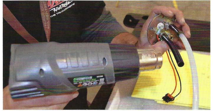
There's a couple tricks to assembling the fuel pump assembly, one of which being that heating the transfer hose will allow it to slide onto the barbed fitting on the fuel pump with relative ease. This type of connection will provide an OE-quality seal that won't leave you stranded on the side of the road.
