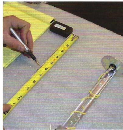
With the depth measurement taken, and the height of the level resistor determined, we can figure how long the float arm needs to be shortened to. The level sender itself is adjustable via-set screws.
