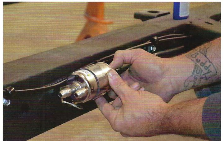
Being as the giveaway car is LS3 powered and won't require any deviation in fuel pressure away from stock, we opted to use a Vette-style filter/regulator assembly. By running the filter and regulator as one assembly, it eliminates an unsightly fuel pressure regulator in an otherwise spotless engine bay, and keeps return hose length to a minimum just the same. It's really a win-win, and all you have to do is find a good spot on the fuel rail to mount it.
