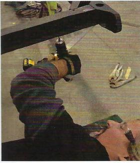
With the tank out of the way, Joe Shinliver of "Trust the Builder" fame drills the mounting holes in the rear crossmember.
