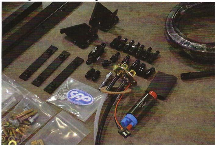
Along with the 29 gallon tank, we're using CPP's EFI fuel kit, which in this case, gives you a in-tank pump, post-filter, Corvette-style filter-regulator setup, and push-lock style fuel hose with AN ends.
