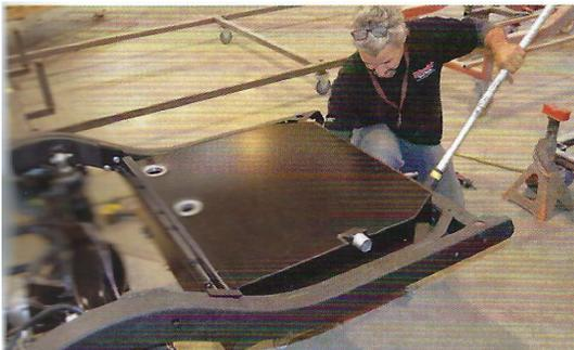
Holes are mounted, tank goes back in now, front first. Again, remember that a few of these steps are done differently, since we still have access to the tank with the body out of the way.
