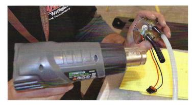
There's a couple tricks to assembling the fuel pump assembly, one of which being that heating the transfer hose will allow it to slide onto the barbed fitting on the fuel pump with relative ease. This type of connection will provide an OE-quality seal that won't leave you stranded on the side of the road.
