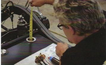
Just like the sending unit, the fuel pump assembly is a universal component that requires roughly the same modifications. Again, make sure these measurements are correct, as incorrect measurements will leave the pickup sock shoved against the bottom of the tank, or too tall to properly utilize
