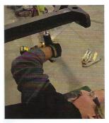
With the tank out of the way, Joe Shinliver of "Trust the Builder" fame drills the mounting holes in the rear crossmember.
