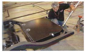
Holes are mounted, tank goes back in now, front first. Again, remember that a few of these steps are done differently, since we still have access to the tank with the body out of the way.
