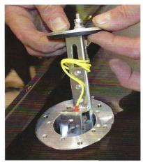
With the sending unit finalized, it gets slid into the tank. If the body was on, you'd want to install your lead and ground wires now, as once you lift the tank in place, they won't be accessible.
