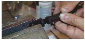
With the filter/regulator mounted, we're onto fuel lines. CPP's fuel kit uses push-lock hose and AN-Style fittings throughout. Assembly is as simply as gets: insert the fitting into a vise, cut your hose to length, and push your hose on. The one-way barbs on the fitting will hold it in place for good. If they give you any trouble, a little heat applied to the hose generally makes them easier to work with
