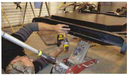
The rear tank mount uses a reinforcement bar for final installation. No worries of pulling through the frame on the rear.
