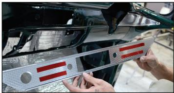
The center will install the same way as the corners, minus the mounting screws, just with a little more tape to hold it in place. Ultimately, the radio post nuts will help keep it in place as well.
