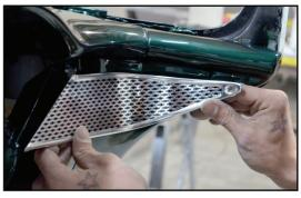
Factory 150 and 210 cars lack the screw hole in the corners of the dash necessary to mount the corner pieces of the dash trim. This is easily rectified
