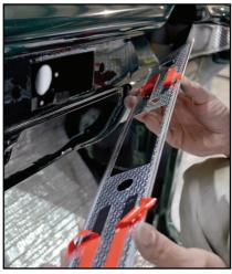
Peel back the tape again, working from the center of the trim piece out, making sure it comes past the edges so you can grab a hold.
