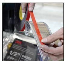
Peel a couple inches of the red backing tape away from the edge closest to the speaker opening,
