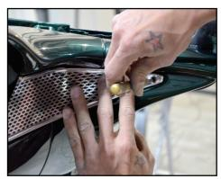
With your hole marked, use a 1/8" drill bit to make your mounting hole.
