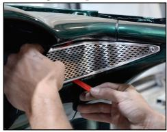
With the mounting screw installed, pull the tape away while pressing on the trim, working your way towards the screw.
