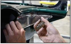
leaving enough to stick out past the edges of the trim, and line it up with the edge of the dash. Once lined up at the edge, press down at the exposed tape, and once pressed down, install the mounting screw provided in the kit.
