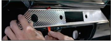
You'll need to pay a little more attention here, as you'll be aligning the radio openings as well as the edges to the dash. Push down on the exposed tape and pull the red backing off, working towards the edges.
