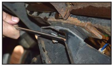
Next, unbolt the core support from the frame mount. If the stock bolts are in place, these are carriage head bolts, so makes life easy. Keep an eye out for the shims when the front end comes off, keeping track of those will make reinstallation easy.
