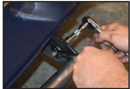
Front bumper (or in this case, push bar) will need to be removed. Unbolt, and stash away accordingly.
