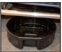
Helpful hint: jacking up the back of the car will force antifreeze in the block towards the front, making for less of a mess upon radiator hose, and/ or engine removal.
