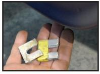
We've come to the first part of the car where traditional body shims will likely be found. The lower shims will space the fender out to match the contour correctly,
