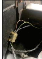
Front light harness is next. There will be connectors both on the passenger side and driver's side. Simply unplug, pull the harness back, and set it up against the cowl, out of the way.
