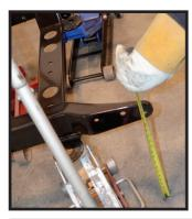
Head back out to check the height on your mount holes. Note the use of the floor jack; this will make nailing the height especially easy.
