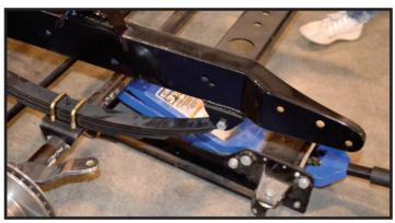
.....then pull up to meet the front leaf spring eyelet.
