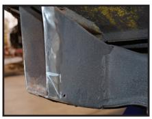
With marks made on the inside and outside indicating the height of the BAG stub, mark back on a 45 degree angle, roughly 1" back until it meets the bottom of the frame. This will be a good starting point for your bottom frame section. You'll trim more later, but this will make it easier to work with, and should ensure you don't wind up having to fill it back in.
