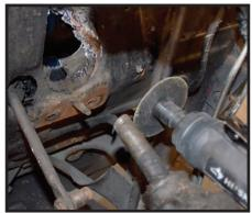
Since the steering box on this one is pretty well shot, and I didn't want the extra work of disassembling all the steering, I chose to cut the steering column shaft to make life easy. This is surprisingly easier than you'd probably think, and only further solidifies that grinding a factory steering shaft into a double-D to use with an aftermarket steering box is a terrible idea.
