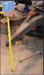
Use a plumb bob to locate the core support lower mounting holes.
