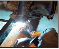
With the outsides and bottoms fitting nicely, go ahead and weld them up completely, as well as the outer part of the top, as you'll most likely
