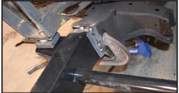
Once your heights are correctly verified, apply more tacks to the inside of the frame rails. This will be sufficient to keep everything in place.
