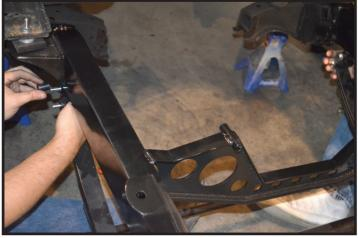
Wheel the axle back over and start reinstall. I find it easiest to attach the shackle end first....
