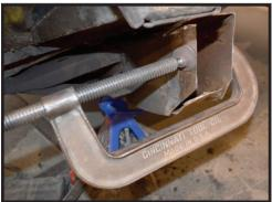
Some large C-clamps will come in handy here; with your cuts made, the c-clamps can be used to push the "flaps" over into position. If you choose to instead bang these over with a hammer, be VERY careful not to scoot the car on the floor or stands away from its initial position. The C-clamps are a much better choice, IMO.
