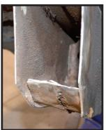
Once the bottom is cut, take a hammer and work the bottom "flap" up to your marks on the side, indicating the correct height for the BAG stub.
