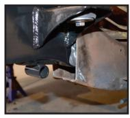
Here you see the distance between the original frame and the new stub that needs to be made up. Looks like our marks are in the ballpark, so time to cut.
