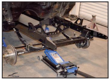
And done! At this point, you'd reinstall the front shocks and steering box, as well as whatever steering column you deem fit. This will come later for this particular car.
