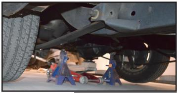
You'll be referencing off the bumper bolt holes in the front frame rails. Keep in mind, these are crucial measurements: If you notice any damage at these areas, IT CAN AFFECT THIS **PROCESS!** The better car you start with, the better product you end up with, so check from the firewall body mounts to make sure your front end is square, or something close to it. This particular car was about as good as it gets for a 65 year old unit.
