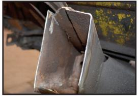
Helpful tip: If using a cutoff wheel, it'll be easier to cut the top corner from the inside of the frame. There's simply not much room up here to the firewall mount on the body.
