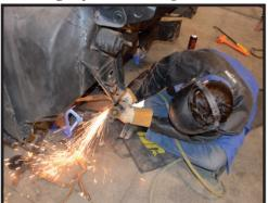
With both sides marked again, go ahead and make the final cuts to the sides.
