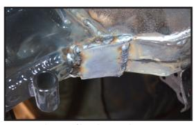
Triangulating/bridging the gap between these two areas will add strength to this stress point, whether you're riding wheelies at the track or hitting potholes out on the streets!
