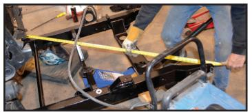
Re-check square again to ensure tacks didn't pull it one way or another. Remember, its easier to grind off a few tacks than it is to cut an entire weld free, so don't be afraid to verify your measurements multiple times.
