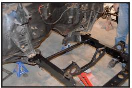
This will be the first of many times you'll trial fit the stub. The first time, shown here, will give some idea how it will all look, said and done. The new frame section slides into your existing frame, so slip it in and give it an eyeball to see if the body mounts are in the ballpark. If they aren't, trimming the frame rails back will be required.
