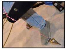
Check your plumb bob marks at all locations. Between this, and checking for square, you should be able to ensure you're in the proper position left to right.
