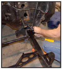
Once you have the stub as far up as it'll go, install the body mount bolt and cushion. More shim may be required here than factory, FYI.
