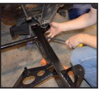
With your marks made, you'll reinstall the stub to verify your marks. Use a pry bar on the bottom side to push the frame up to the top as described a few steps back.
