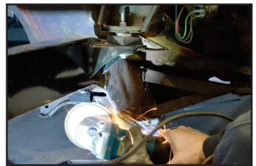
Break the flapper back out to clean up the mounting surfaces for the plates. Again, cleaner the surface, the better the weld.
