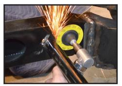
With the stub finish welded, the round reinforcement bar can be cut out. It's just tacked in, so grind the spot welds out and give it a whack with a hammer and it should come free.
