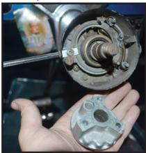
Hub is off, next we go under the dash....My With the column support loose, slide it down the tube, and rotate it so it clears the factory shifter arm(s).
