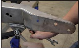
The stub will need to be broken down to just the bare rails, at any rate. Front leaf spring bolt nuts are first.
