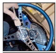
The column needs to be removed (and won't be reused), so we start at the top with the steering wheel. Dig that original Superior 500 flake! Next, remove the lower column cover and column support.
