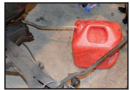
Helpful hint: Gas will find the lowest point in the system (thanks to gravity). If you forgot that you had a half a tank of fuel (like I did), draining it and removing the main line, as well as the brake lines, before cutting and welding up front is a solid idea.
