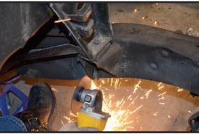
support the front end with a floor jack, and fire up the cutoff wheel. I started outside first on both sides, then bottoms, then insides, then tops.
