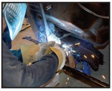
Double checked and triple checked, it's time for the first welds. Tacks on the upper corners of the inside are the first.
