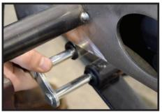
The shackle itself can then be removed, along with the bushings, and set aside for safe keeping.
