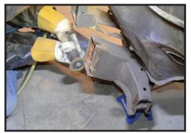
I started top to bottom with my cuts. For the bottom, I slit past my mark on the side, on each side, knowing it'd be fairly easy to weld up and finish off it necessary.
