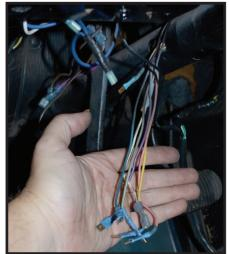
Either way, it needs to be unplugged to remove the column. Also note the tachometer has been removed from the column as well. Don't forget, if you're so equipped. This may require some persuasion, depending on how long it's been in place, or how many layers of paint/ grime are on it.
