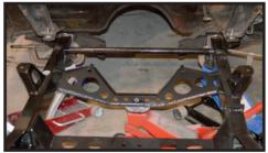
Once your body mounts are bolted down, go ahead and reinstall the C-clamps on both sides.
