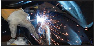
With your measurements verified one last time, go ahead and fully weld the insides of both frame rails, rolling over onto the upper section, as well as a tack or two to the outer sides.
