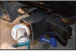
A grinder with a flapper disc is my weapon of choice for cleaning up both inside and outside the frame rails, as well as the painted areas of our new stub where welding will occur. The cleaner you get this metal, the cleaner it will weld.
