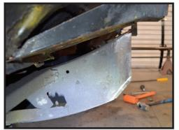
Now, as mentioned before, the initial mark will likely be short, and will require more trimming. So, once the lower flap meets your bottom-of-stub measurement on the side, you can re-mark to match the actual cut and angle you wind up with.
