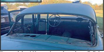
Done and done! Now you're ready to clean off all the sealer used, and move forward with body work or install your new glass. Keep an eye to the tech section here, once this dude is in color, we'll be showing you how the glass goes back in!
