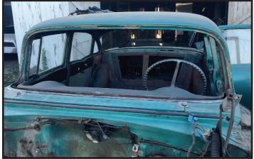
....and just like that, windshield out! On top of a pure glass or seal replacement, windshield removal for proper paint and bodywork is a must, especially if you plan on painting the dash.
