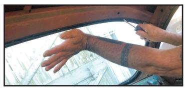
outward. On a hardtop or '56/'57, you'll need to be extra careful here as not to damage the headliner.
