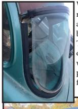
With part of the seal lip removed, and the proper amount of pressure, you should be able to get a corner started. The 64 year old rear seal on this one literally deteriorated as we worked our way around. Apply pressure across, starting in the free corner.
