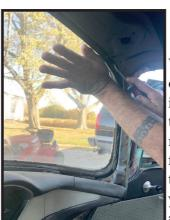
With the garnish mouldings out of the way, the pick tool is inserted into the lip on the backside of the window rubber. Work back and forth from the middle to the corner of the windshield you're focusing on while applying pressure outward.
