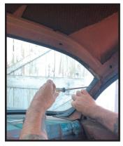
Rear window removal mimics the front to start. Garnish moulding removal is first if you own a '55 sedan, be it two or four door. If you have a 210 or Bel Air, doing so would give you access to the studs for the outside corner mouldings for the rear window trim. If you have a '56 or '57, garnish
