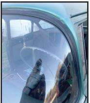
As you can see, the windshield was heavily scratched from worn wipers, pitted heavily, and hazy from delaminating. The miles I put on the car last season were tough looking through this, especially in the hours where the sun was low in the sky. Time to go!
