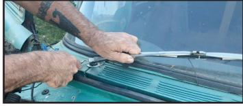
window stainless to remove. But if you have a 210 or Bel Air, after the wiper removal, stainless removal would be the next step. Corners off first, and then lowers. The upper trim installs into the window rubber BEFORE installation, and is not able to be removed with the
