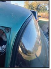
Push, push, push! Sooner than later, you'll get one corner free from the body. Keep in mind, the glass is more resilient than you think, so don't be afraid to apply some real pressure. Once your corner is started, you can apply pressure across the upper section of the windshield, and the back lip of the window rubber will work its way away from the body.
