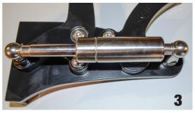
end of the strut, and install them shaft-side down. Don't try to collapse them by hand; you'll need the leverage of the hood in order to do so, as this is how the hood stays up. A word of advice: don't install the wire keepers at this time. You'll likely need to remove the strut in order to adjust the hinges
