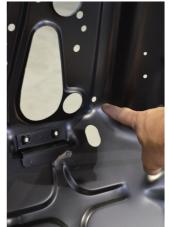
4. The bottom left hole on the bracket aligns itself with a factory hole next to the recess on the firewall. This gives you your reference point for the other three holes to be drilled. Bolt one through, hold in place, and drill through the holes in the bracket.
