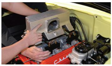
Setting the plenum on can be a two man job, with two hoses and four injector rails to manage. Having a buddy handy will make quick work of lining everything up. Finally, starting to look like something!
