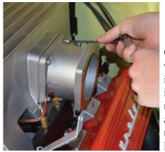
Once your vacuum fitting is completed, install the throttle body adapter using the supplied hardware.
