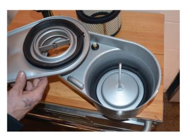
The LS Classic air cleaner comes with a white paper filter element with a glue-on weatherstrip seal.
