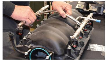
Go ahead and remove the throttle body and the fuel rails/injectors. Unless you're doing significant engine upgrades at the time of the intake manifold, the stock injectors and throttle body supplied with your engine, such as our 376/480 crate motor, will be just fine.
