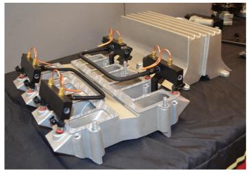
With the upper plenum removed, you can see the feel lines to each injector and rail. With the Corvette-style filter/regulator assembly we used on our '57, the return comes off the assembly itself, so the fuel rails are "dead headed", meaning we feed both rails, but don't return from them.
