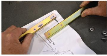
11) Moving on to the link arms, when assembling the link halves use the longer pair of holes for the nuts and bolts.
