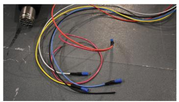
6) Wiring the motor and switch before assembly can be helpful because sometimes it can be difficult to install the wire harness if everything is already in place.
