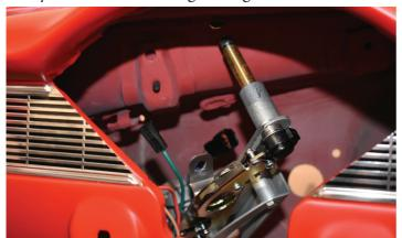
9) You'll want to place the locator tab on the firewall fitting. There should be a hole up and to the right of the locator tab. This is where the shaft will fit in. Attach the assembly against the firewall using the  $5/16-18 \times 1/2$ " hex bolt. If you have a gap between the locator tab and the firewall fitting you will want to bend the locator tab a little bit more.
