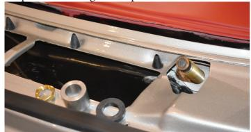
8) From the outside of the car you want to place the rubber washer, the aluminum spacer that is 13/16" long, and the 5/8" nut on the pivot bar. When tightening the nut, you want it to be snug, not tight.
