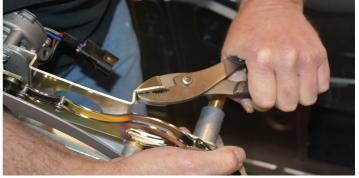
want to bend the locator tab out about 30 degrees. Doing this before assembly will be much easier than doing it right before instillation.
