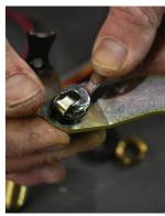
13) Piece together the extended end of the long link to the passenger side using the given bushing, washer and clip. Be cautious when installing the J-clips, they can be easily lost. We recommend using a 1/4" wrench to push down and put the J-clip in place. Make sure that the lever on the passenger side pivot shaft is at 10 o'clock.
