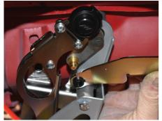
16) Attach the link arm to the brass pin on the driver side drive assembly as we did to the passenger side with the shoulder bushing facing toward the pivot fitting.
