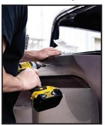
Grab your drill and some self-tappers and go to town attaching the firewall to the upper cowl and cowl shoulders to hold it in place as you weld. Remember, less gap, easier to weld, so manipulate if you must!
