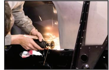
You'll want to notch the toeboard for the firewall to slip into once left – right orientation is determined. This will keep it centered.
