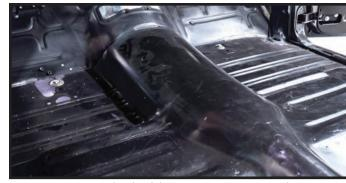
Now, to move to the inside. As you can see, the factory transmission tunnel isn't much of a rise. It's not hard to see how any kind of a taller transmission would be a problem. For what it's worth, any of the GM 4-speed automatics or 5 speed manuals will fit the tunnel without modification.
