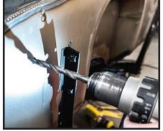
With your firewall completely welded, you'll head to the inside of the car, take a small drill bit, and drill through the lower hood hinge captive nut on the firewall. You can only do this
