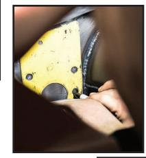
With the template against the recess, mark the four mounting holes for the master cylinder. Grab the small bit you used to drill pilot holes for the hood hinges, and do the same for these holes.
