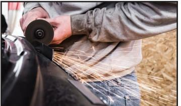
As shown, Dillon likes to notch straight down, and then cut over, as it gives a reference of where the upper cowl is and keep from leaving wild excess to trim back.
