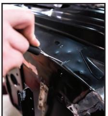
With the braces loose, take a scribing tool and mark the location of the hood hinge holes on the upper cowl area. The HRD firewall doesn't have these holes pre-located, and we'll need to drill them after the fact.
