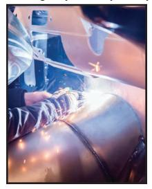
From there, you can work the tunnel all the way around, welding small sections at a time to keep warpage to a minimum. Granted we're not doing bodywork here; it'll simply keep your tunnel as straight as possible while working.
