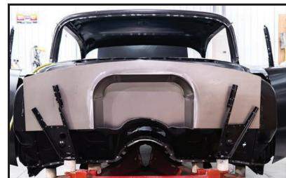
With the toeboard notched, and the recess trimmed. your firewall should fall neatly into place. You'll notice again, that HRD gives you plenty to work with at the top as well. Remember, we're working with cars that were built with some wild tolerances, and these parts are made to be as "one size fits all" as possible. The passenger side will typically need a smaller amount more trimmed off than the driver's. This is normal, so don't worry that it's not level!
