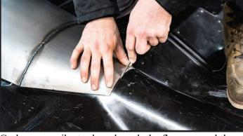
Grab your scribe tool, and mark the floor around the outer perimeter of the trans tunnel. This is especially easy with the EDP on the new floor pans, as it shows up well. If your floor is a touch dingy, simply use your favorite marking tool.
