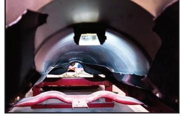
With the top welded, it's time to head to the bottom! A few relief cuts will need to be made to bring the floor up against the transmission tunnel.
