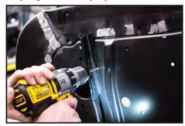
The firewall braces need to be removed and drilling the spot welds is by far the easiest way to do so. Just like doing the floors, a 5/16" drill bit is the weapon of choice here. They should be fairly visible.
