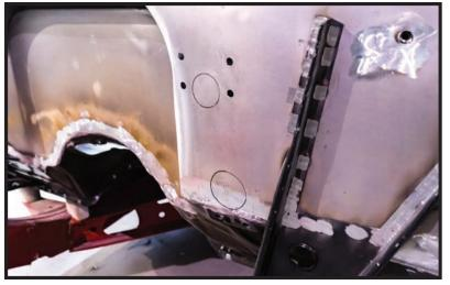
Remove the template, and you'll see both the holes for your brake and column clearly marked. Time to make more holes!
