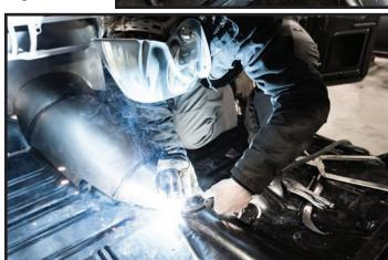
With a small amount of pressure applied, tack the tunnel in place in a few spots to prevent it from "walking" as you work your way around.
