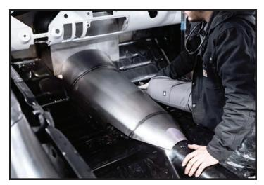
And with the HRD Transmission tunnel laid in place, you can see this is world of difference! Nice thing as well, HRD offers this tunnel cut for a factory firewall as well, for those not doing one of their recessed setups.
