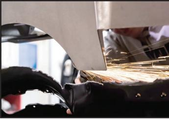
The recess is purposefully left long, so trimming will be required here for perfect fit to the toeboard as well. Simply measure twice (or four times) and trim away.
