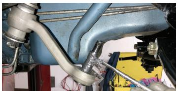
As with many of the suspension pieces, a generous helping of silicone grease on the idler bushing is a good idea and will keep all pieces moving free. If you feel like upgrading this area even further, have the guys at Woody's add on CPP's idler bearing conversion kit (part number CPP-5557IBC).
