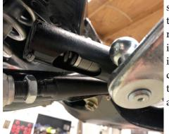
screwdriver the run the retainer out in order to install the drag link to the pitman arm.
