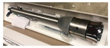
Since the steering linkage is now complete, we're moving along to our column. These new columns, available from Woody's, feature a 5 position tilt, a 9-bolt steering adapter (but will accept any OE wheel or applicable 3-bolt style) and available column shift option. They come in chrome, black powdercoat, and bare steel, which we chose so we could keep the Del Ray looking as stock as possible inside.
