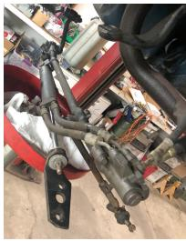
With the ram loose from the frame, you can drop the entire drag link assembly down. No need to take it apart further, nothing from this setup will be reused, even if you have a manual steer car to start with.
