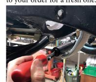
With everything in place, you'll re-install the retainer, preloading the spring inside and re-install the cotter pin. This area is adjustable for variances in the pitman ball and for wear.
