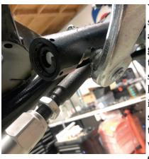
You'll move the steering linkage back and forth in order to get the ball in and over towards the passenger side in its intended location. Note: There is indeed a dust shield/ seal used here around the pitman arm ball, we simply didn't have one on hand, since our
