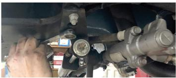
Next comes the ram bracket. Wildly different from a modern power steering setup, the OE Power steering configuration used a directional control valve and a hydraulic ram to assist with steering effort. This setup is large, above anything, and can be extremely expensive to have rebuilt if problems present themselves. This one was in good shape, but with all the modern amenities this car is getting, the step to a "normal" power steering setup was a no-brainer.
