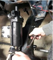
Installation of the box is extremely straight forward. It bolts in the factory position, using provided hardware. As I mentioned earlier, the box is threaded, so it no longer uses the factory carriage bolts.
