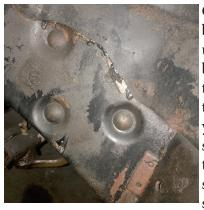
Original steering boxes were thru-bolted using carriage-head bolts. You won't need them, the new box is threaded, and provides you the hardware to do such. Simply remove the bolts, and angle the steering box and shaft so you can remove it.
