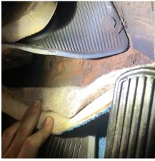
The IDITIT mount uses the factory outer column support nuts in the toe board, only this time on the inside, shown here.
