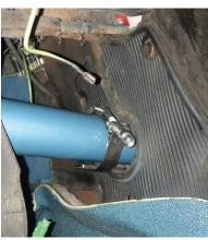
With the column in place, affix the factory upper column mount, and use the supplied t-bolt clamp to bolt the column down to the support.
