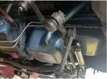
With the tie rods loose on both sides, you can simply swing them down and out of your way. Since the Ridetech kit is complete, there's no need to worry with extra disassembly of the inners or idler.
