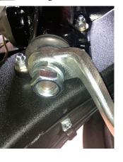
The center link attachment point consists of spring loaded cups that fit around the ball on the pitman arm. You'll remove the cotter pin, and use a flathead
