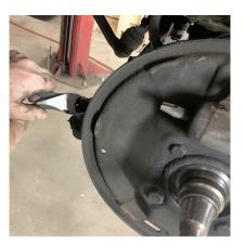
so cotter pins get pulled right away. I'm a fan of using a pair of sidecutters to get a good bite and leverage against the castle nut. New tie rods will come complete with cotter pins and castle nuts.
