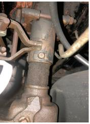
for wheels/adapters. Use a steering wheel puller to remove whatever wheel you have, unplug the harness at the column, remove the upper bracket, and slide the column off the steering shaft.
