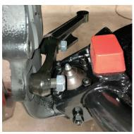
New hardware for the steering arms is provided, but some brands of drop spindles, such as the CPP units, use a flush mount allen bolt instead.
