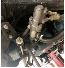
bolts onto the pressure control valve. Spinning the nut back off the stud, but not all the way off, and giving it a couple taps with a hammer should set it free.
