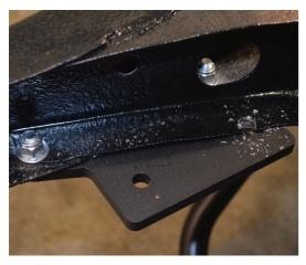
On our '56 wagon test mule, the frame bracket for the sway bar indexes off the rivet in the bottom of the front frame horn. Once the rivet is ground down, you can drill the hole to the required 3/8", bolt it in place. Note the use of clamps to ensure everything stays put.
