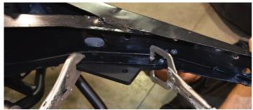
Your third bolt will bolt through the frame, the bracket, and the sway bar mount as well. Using the mounting bracket as your guide for the drillbit will help keep things lined up.
