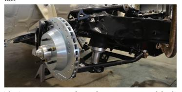
The StrongArm control arms have a mounting tab built onto them, made specifically for the MuscleBar. Again, stock control arm guys, the StreetGrip bar comes with mounting tabs that are easily installed to your control
