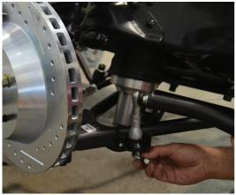
Once your PosiLinks are assembled onto the sway bar, they are then bolted through the control arms. Simply bolted through, no pesky bushings to hold together.
