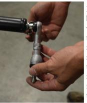
Ridetech's PosiLink Sway bar endlinks are part of what sets this kit apart from the other sway bars on the market. Think of these as miniature tie rod ends on the end of your sway bar; no binding, no unwanted noise, and much longer life than the average bushing setup. They simply thread
