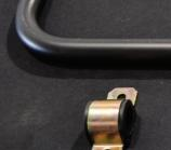
The MuscleBar sway bar installs much like all other sway bars, but utilizes a PosiLink as opposed to the standard pedestal mounts more commonly used. This allows for more articulation and better, fluid movement from the sway bar.
