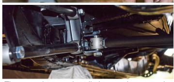
The control system installation requires mounting the air tank, compressor, valves, lines and control module.
