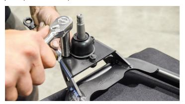
NOTE: the top ball joints on RideTech Strong Arms are taller than stock, this allows for improved camber angle so that when the suspension is under a load in a corner the wheel stays straight up and down so that you retain the maximum amount of contact patch from your tire.
