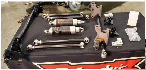
When installing the 4-bar rear suspension you must weld the brackets to the rear end housing. It is very important that you set the 3 degree up position of the pinion angle.
