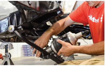
With the upper and lower control arms installed, the front Shockwave shocks can be installed. The shocks are adjustable depending on each owners ride preference. To install them, you must remove the adjuster knob, then reinstall it once the shock is in place.
