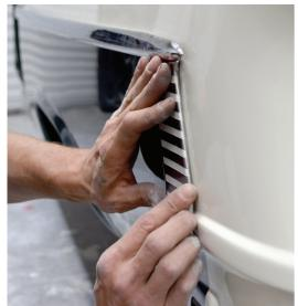
The lower paint divider has contours built into both ends, so fitment \*should\* be pretty straight forward. However, again, some alignment may be required of any and all pieces in order to fit as nice as you'd like it to. Splitting the difference can be taken into account here just the same. The studs for the clips are easily accessed on the backside of the quarter panel.
