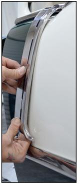
As with the other mouldings, move your trim clips to correspond with the holes, then go ahead and set the upper paint divider on the body. Don't bolt it down just yet.
