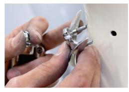
...and since this car will wind up with an LS3 as the build progresses, the decision was made to add the factory V8 emblems under the taillights for additional flair. With careful measurement, taping, and drilling, these emblems can even be added after the fact to a done car.
