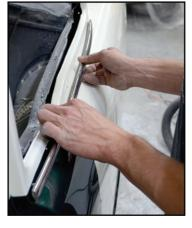
With everything aligned to your liking, go ahead and insert the moulding, and tighten from the inside using the nuts supplied in the kit.
