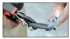
The clips aren't \*ridiculously\* tough by any means. A set of tin snips will be sufficient to cut them, as shown, but your favorite cutting tool can be used.
