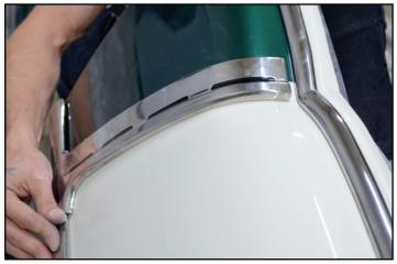
There will be some adjustment in how the paint divider can sit on the car. Line it up with the quarter spear, and make sure it is even up top, then go ahead and cinch it down.
