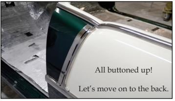
When using the popular two-tone including the roof and the quarters, a lower, or rear, paint divider (DAN-152) is a must. The same clips we used for the uppers, can be used at the rear
