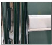
The door opening is a perfect point of reference. Obviously, you don't want to leave this gap too wide, or the quarter moulding loses continuity to the door point or be so far over the edge it makes contact with the door. Once it is where you like it, attach the mounting screws from the inside, both in the access panel area if the quarter window, and on the inside of the quarter panel as you go back.
