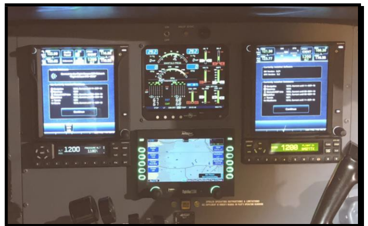
Garmin Touchscreen Glass Panel with Avidyne MFD, JPI Digital Engine Monitoring & L-3 Standby Instruments
