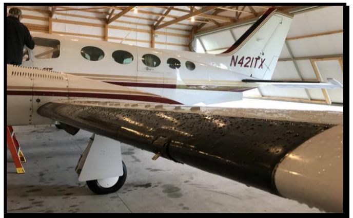
So Many Enhancements: Spoilers, Hubcaps, VGs, & Aft-Body Strakes
