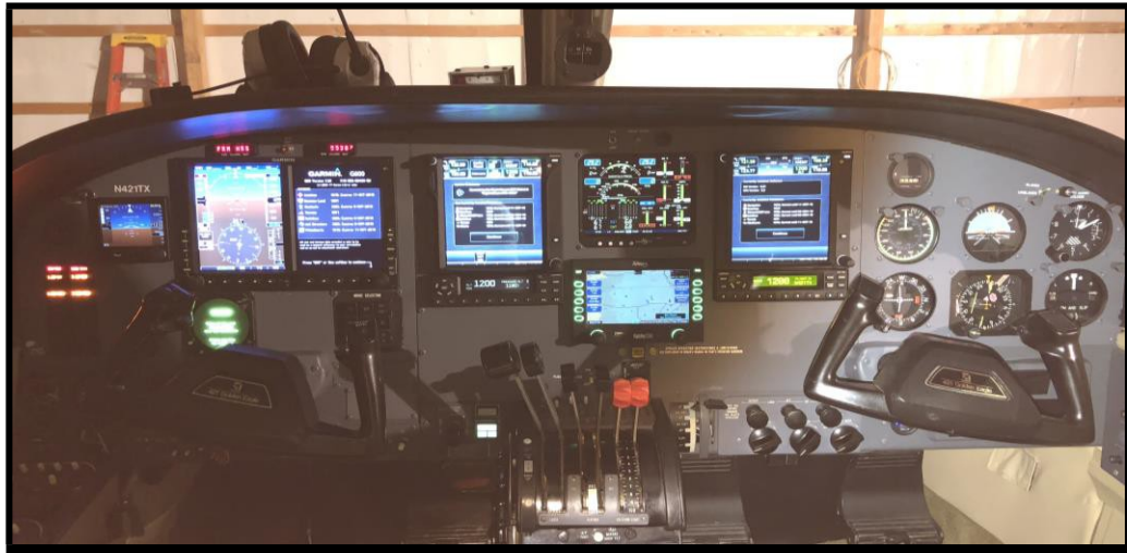
Garmin Touchscreen Glass Panel with Avidyne MFD, JPI Digital Engine Monitoring & L-3 Standby Instruments
