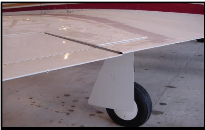
So Many Enhancements: Spoilers, Hubcaps, VGs, & Aft-Body Strakes
