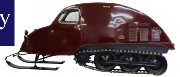
Bombardier "B7" -The B7 model was the first snowmobile mass produced by L'Auto-Neige Bombardier. It was designed for commercial use and could carry up to seven passengers. Unlike the regular model, it had no side windows. Starting in 1940, the B7 was equipped with a new suspension system for better traction; spoked wheels were replaced with solid steel wheels, thus eliminating the risk of snow accumulation in the system.
