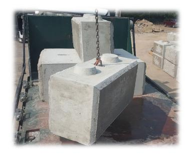
Each pick point is comprised of a "cupped out" region on the top of the block with either an imbedded rebar cutting across or a u-shaped lifting loop. Either type of pick point can be hooked onto with a chain and hook assembly.
