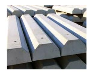
All parking stops are 5.5" tall, 8" wide at the bottom and 4" wide at the top and have two 0.75" diameter holes for pinning the parking stop to the ground. There are two pieces of #4 rebar placed inside the stops during production to add tensile strength. Our 6', 7' and 8' long stops weigh approximately 225 lbs, 275 lbs and 325 lbs respectively.
