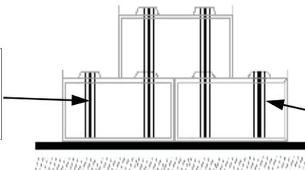
Internal bollard tubes are precast into each block.
