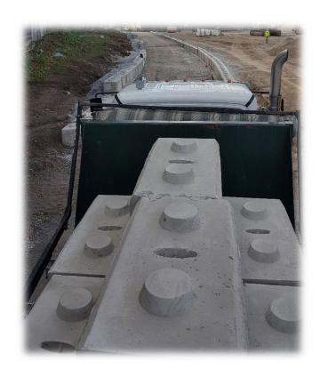
Our typical delivery is 40,000 pounds of product which equates to between 16 and 22 blocks per load depending on block type, size and finish.
