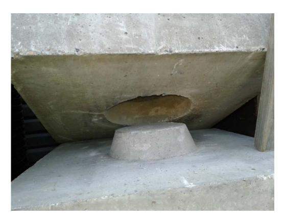
Figure A-2. Round cavity at the center of top block and knob at the center of bottom block.
