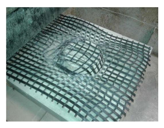
Figure A-5. Abrasion and rupture of SRW-11 geogrid ribs at the completion of a test.
