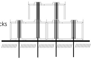
1 1/2" diameter Internal Bollard Tubes are precast into each Block
