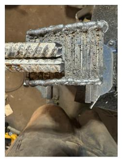
Because this is a heavy billet, I am going to attach two pieces of rebar instead of one so that when they get they white hot there will be more support. I cleanup the ends on about a 45 degree angle and this seems to give me better welds to the billet (but again, I am not a welder, your mileage may vary). I then tack the two pieces every 6" or so to give it a bit of rigidity.
