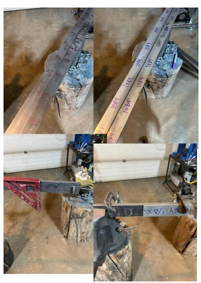
I only have an angle grinder to do all my cutting with, so I clamp the steel together to create 5 1/8" pieces allowing 1/8" for the cut. Getting maximum use of the 4' length of steel.
