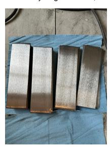
I used to use latex gloves when handling the steel to avoid finger oils from getting on the clean steel, but now I am just careful to only handle the edges once they are cleaned.
