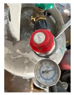
Your forge will be different, but for setting the initial tack welds, I run a propane rich flame. The gauge says 5lbs of pressure, however, that is not accurate because of the ribbon burner build. My gas runs to a hole drilled into a end cap. I cant remember the size, but I tried the .035 mig tip and it was way too small. All this to say, your gas settings will vary.
