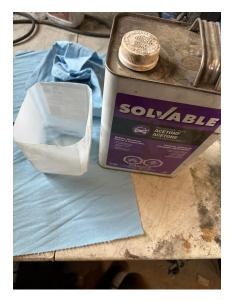
I completely submerge the steel, then wipe them off. Making sure to keep track of the stacks at this point. I make a mark on the shop cloth with the appropriate color because the acetone will take off the edge color now.
