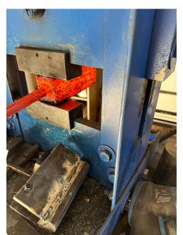
I use the 12T press with flat dies, but barely kiss the billet on the first pass. Just enough that I can see the layers move together. I could probably do more, but here caution is king. Rushing this step has ruined more steel for me.
