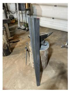
I start by making the Damascus for the outer layers. My target is 120-160 layers on each side. I will then use a 3/16" 1084 core with .4 - .6mm of copper depending on the desired thickness. This post will cover the creation of the Damascus.
