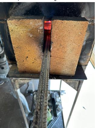
The Billet is heating up. I like to get it REALLY hot before I set the welds. I probably sprinkle with flux starting too early and then every 4-5 min with light sprinkles of flux remembering to do the ends of the billet as well
