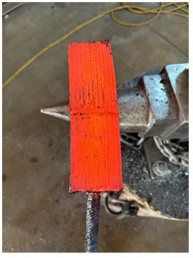
Before we go too far, I need to grind off the mig weld in the middle of the billet as well as the ridges from the layers. The different layers of steel were ~2". But not exact. So when I square up the billet, I dont want one of the wider layers folding over and creating a cold shut (piece where the steel did not weld)
