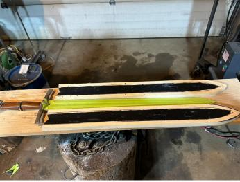
After the felt setup, I then used wood glue to glue the two halves together and shaped by cutting and sanding so that the wood approx  $\frac{1}{4}$ " thick. I used my calipers to continually check.
