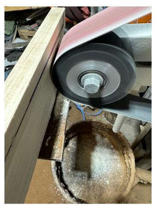
I then used my 2x72 grinder with a 2" wheel to grind out the hollow.
