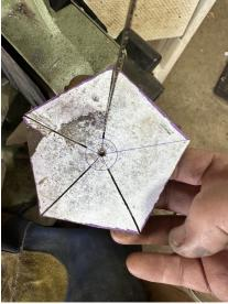
Drill out the center holes with a 1/8" drill bit while the paper templates are still good so that you know where the center is. We are going to make this bigger later, just dont want to loose center once the paper burns off.
