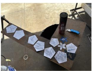
Cut out all of the shapes with an angle grinder or a band saw. I just got a bandsaw it took me ¼ the time that the angle grinder did. Once all of the shapes are cut out, cut the lines from the corners to the center circle
