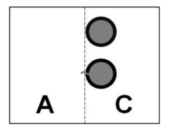
Both of the above rounds are scored as "C" hits because neither the bullet hole nor the grease ring break the perf. Radial tears such as the one on the bottom round do not count.
