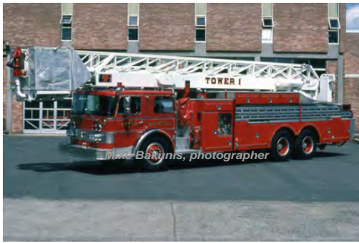
Grumman subsidiary 1988 refurb - Simon-Duplex cab
