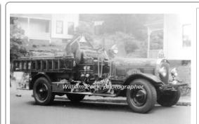
Identical trucks delivered except for pump size - 750 & 600 gpm. Entire department motorized. These two and aerial cost \$41,000. Del 3-1-1922. Painted 2-7-1922
