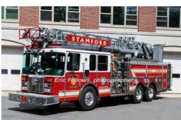
2000 gpm 600 gal tank rear-mount - 75'
