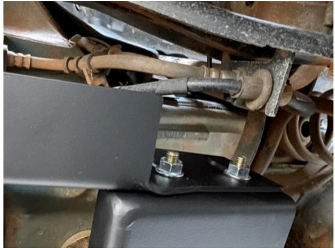
Repeat this procedure with the right front drag hanger. Use a 13mm wrench to tighten the two flange nuts. Do not fully torque them yet. Just make them tight enough to firmly hold the plates in place.
