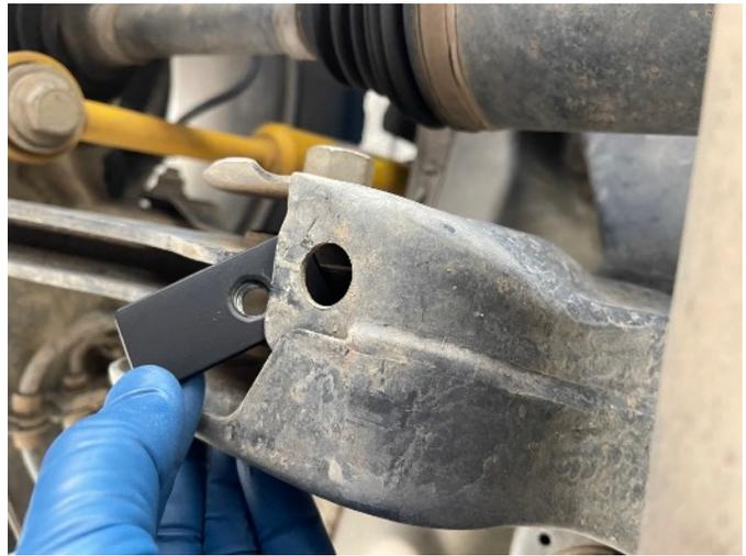
Using the tips of your fingers, maneuver the nut-plate so that the bolt hole is situated directly behind the hole in the toe-link mount, as shown in the picture. A Phillips screwdriver is helpful in aligning the hole.
