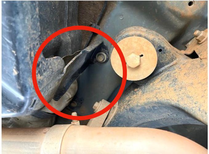
Use a 15mm socket on a long extension to remove the bolt that connects the fuel tank skid plate riser to the unibody.
