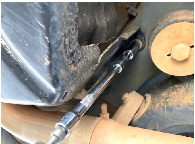
Install one of the middle hanger brackets over the hole exposed by the bolt you just removed. Thread the bolt back into the uni-body to fasten the mid-hanger bracket into place. The middle hanger bracket should nest inside the fuel tank skid-plate riser and the “zig” in the bracket should point away from the exhaust pipe.
