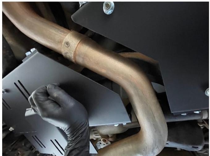
Once the bottom edges of the main & left toe plate are even, use a 13mm wrench to tighten the four flange nuts on the exhaust hoop to keep them aligned. Do not fully torque just yet since you may need to come back and adjust the hoop. Just make sure the nuts are tight enough to hold both plates even with each other.
