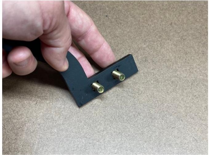
Push the protruding threads of the two carriage bolts through the slots on the front of the left toe plate as shown. In this configuration, the hoop will be on the inside of the front flange of the toe plate as shown in the picture..
