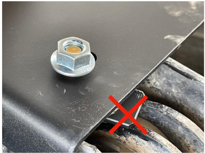
Position the pre-welded studs on the outer, left side of the toe-plate through the slots of the left front drag hanger. Use two M8 flange nuts to hold the drag hanger in place but do not tighten the nuts.
