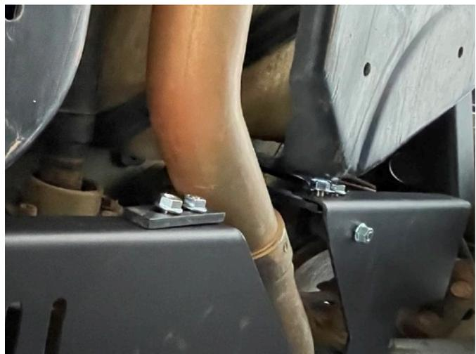
On the right side flange of the main plate, pass the two studs through their corresponding slots on the front-right drag hanger bracket. Loosely thread two M8 flange nuts onto these studs to hold the drag hanger bracket in place. Do not fully tighten these nuts since you will still need to adjust the position of the main plate.
