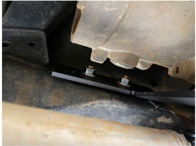
Next, move to the front drag hangers. Choose a side and completely remove the M8 flange nut. Be careful not to lose the M8 washer!
