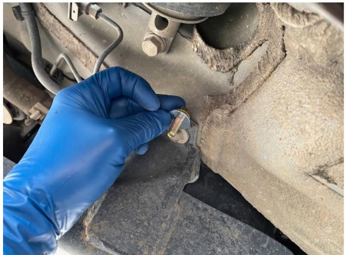
Push the rubber isolator on the right drag hanger bracket onto the thread of the M8 bolt.
