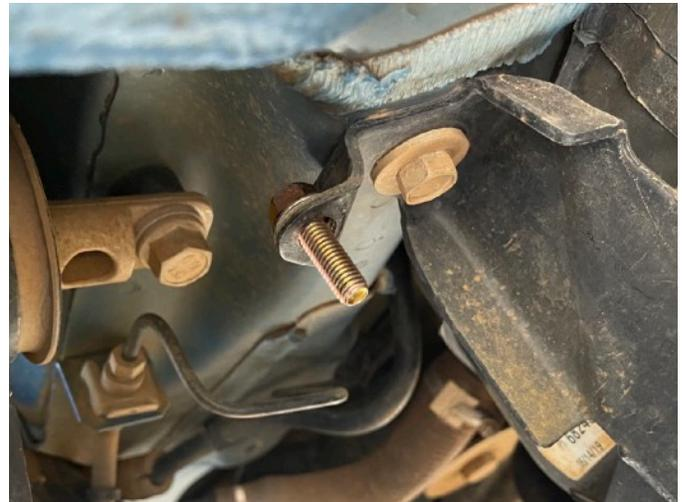
Place one of the M8 washers over the bolt threads and hold in place.
