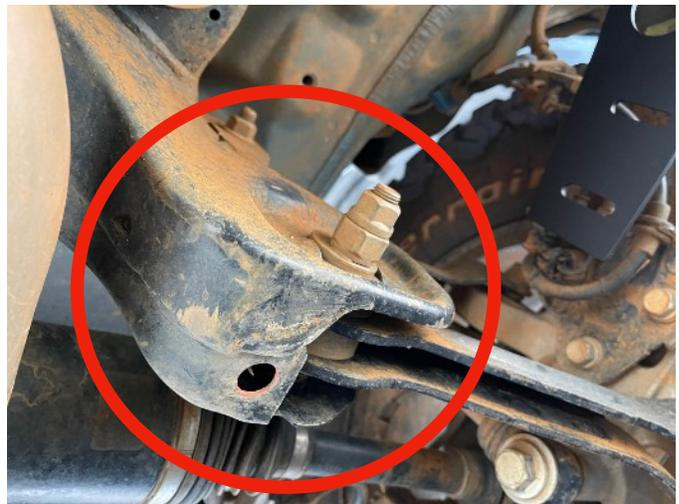
Slide the nut-plate into the toe-mount cavity. The nut welded onto the nut-plate should be facing up and should be inserted first, as shown in the picture.
