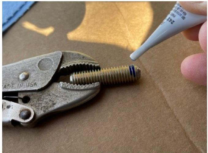
Thread the stud into the nut-plate. It helps to insert one of your fingers into the toe-mount cavity to hold the plate still and provide back pressure while you are doing this.
