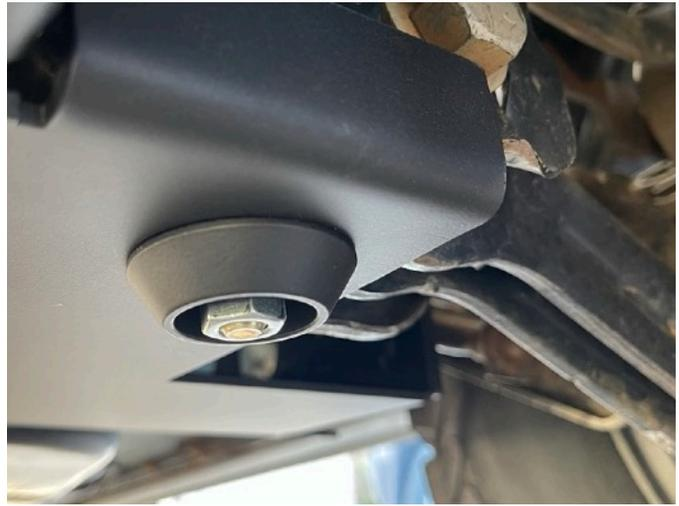
Lastly, move on to the flange nuts for the exhaust hoops and front drag hangers. Ideally, torque them to 22 ft-lbs (29 Nm). If you can't fit a torque wrench into the tight spaces, use an 8" wrench and tighten them as firmly as possible without banging on the wrench.
