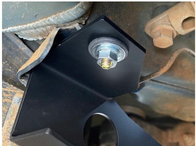
Next, move on to the middle hangers. One at a time, remove the flange nut, place two drops of Loctite on the threads of the M8 flange nut, then tighten the nut firmly, but not excessively, with an 8" wrench.
