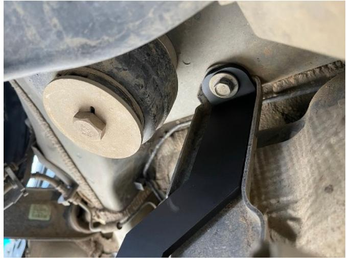
Repeat this procedure for the rear of the right fuel tank skid plate. The riser for this skid plate is more exposed and easier to reach than the one on the left side.
