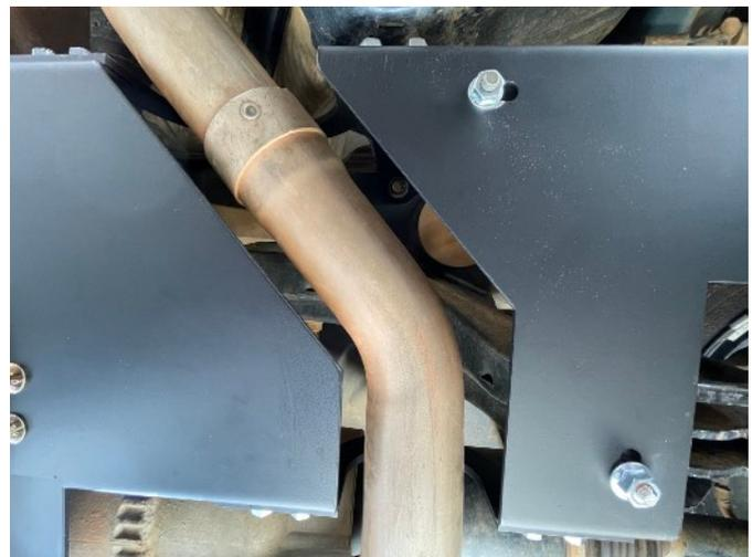
Next, align the bottom edge of the left front drag hanger with the rounded edge of the left toe plate. Use a 13mm wrench to tighten the two flange nuts. Do not fully torque them yet. Just make them tight enough to firmly hold the plates in place.
