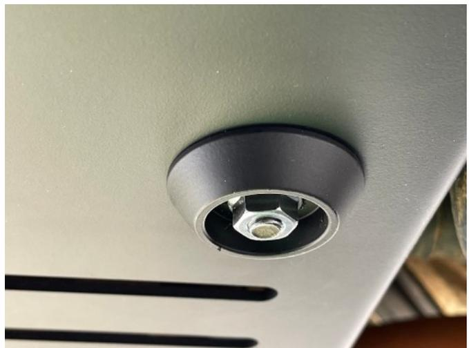
Now move on to the rear hanger and perform a similar procedure. If using bolt-head protectors, remove the flange nut and place it over the stud before tightening the flange nut.
