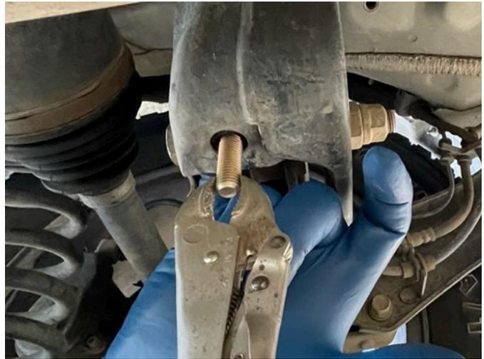
Once the stud has been threaded into the nut-plate, slide one of the thick spacer washers onto the M10 stud and then push the retaining clip onto the stud.
