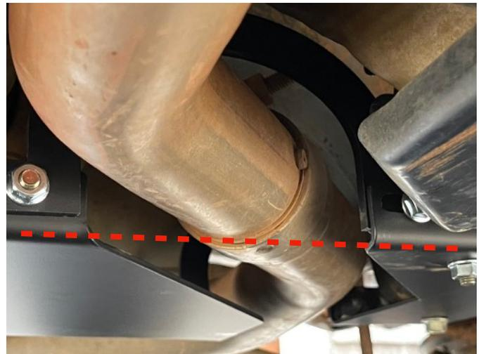
At this point, check to make sure that both the main plate and the left toe plate are more-or-less symmetrically positioned around the exhaust. Also make sure there is at least a finger-tip worth of clearance around the exhaust pipes and both the front and rear exhaust hoops. Adjust the position of the hoops and plates as necessary.
