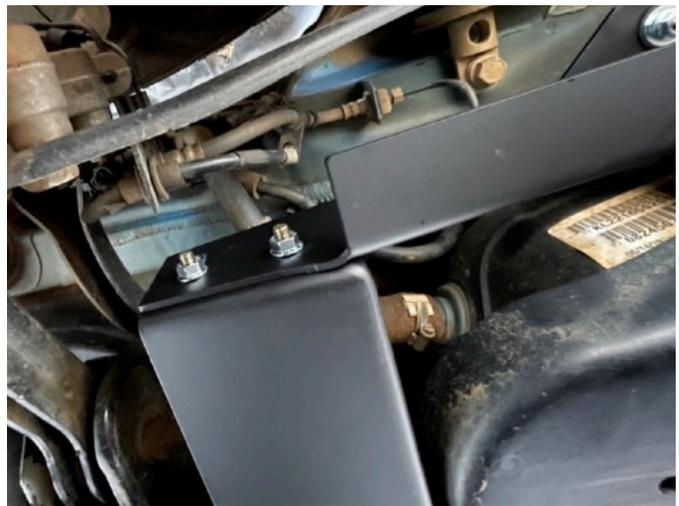
Lastly, use a 15mm socket wrench to tighten the two toe mount flange nuts. Do not fully torque them yet. Just make them tight enough to firmly hold the plates in place. Be careful not to let the nut-plates rotate and interfere with the toe control arm when doing this.
