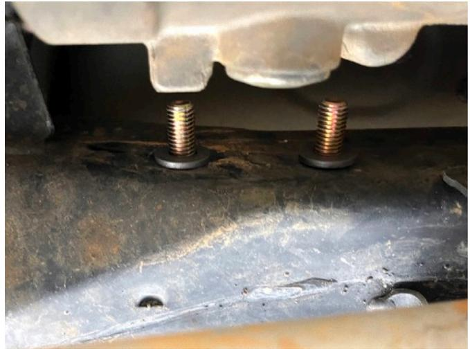
Place the rear hanger bracket over the two M12 bolts. The leg of the bracket that hangs down is positioned towards the center of the vehicle.
