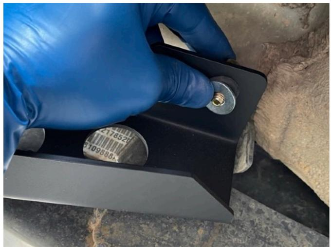
You should NOT fully tighten the nut at this time, Just thread it on by 1-2 turns and then let the entire bracket hang loose. You will come back and secure it later.
