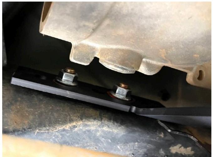
Place the thick spacer on the stud at the end of the leg that hangs down. Press the supplied retaining clip onto the threads to hold the spacer in place.
