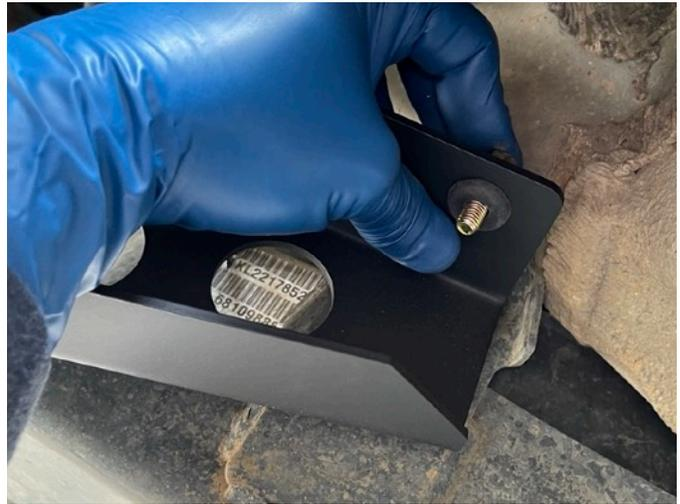
Slide the other M8 washer over the threads and then secure the entire drag hanger bracket with an M8 flange nut.
