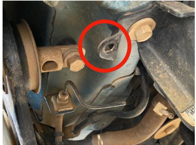
Thread the M8 flange bolt through the auxiliary mounting hole in the fuel tank skid plate riser as shown in the picture.
