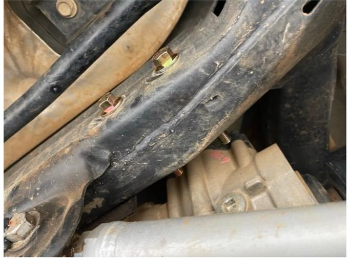
Place the two thick M12 washers over the threads of the bolts in front of the crossmember.
