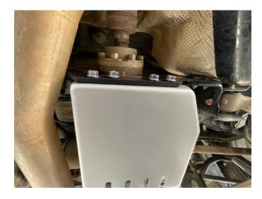
Carefully raise the rear of the diff guard so that the two bolts protruding from the sub-frame crossmember are inserted into the two slots at the back of the diff guard. Be careful not to push these bolts back into the hollow crossmember, since retrieving them can be quite difficult. Once the bolts have been inserted through the two slots, finger-tighten two serrated, flanged head nuts onto the bolts so the diff guard doesn't fall.
