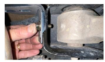
Thread a serrated, flanged nut onto the bolt. Finger tighten it enough to keep the side bracket in place but not so tight that you can't slide the bracket along the slot.
