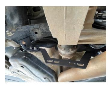
The cross bracket connects to each side bracket using two M8x1.25 25mm carriage bolts. These are the longer of the two carriage bolt sizes provided in the kit. The cross bracket goes in front of the side brackets and the carriage bolts are inserted in front of the cross bracket.
