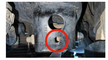
Position the bracket so that the long slot sits over the small hole and that the 90° bent face of the bracket is towards the front of the vehicle.
