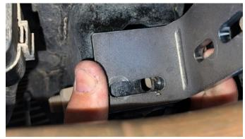
Insert a flanged hex head M8x1.25 20mm bolt through the slot and control arm hole.
