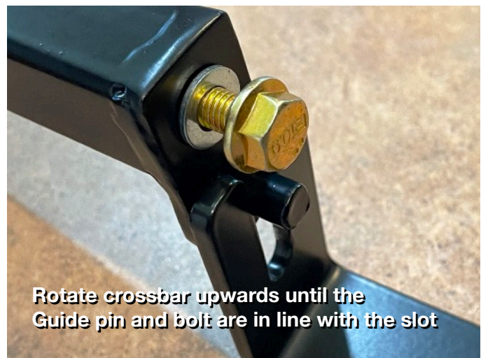
Insert guide pin at an angle (90 degrees in this photo but it can be less)
