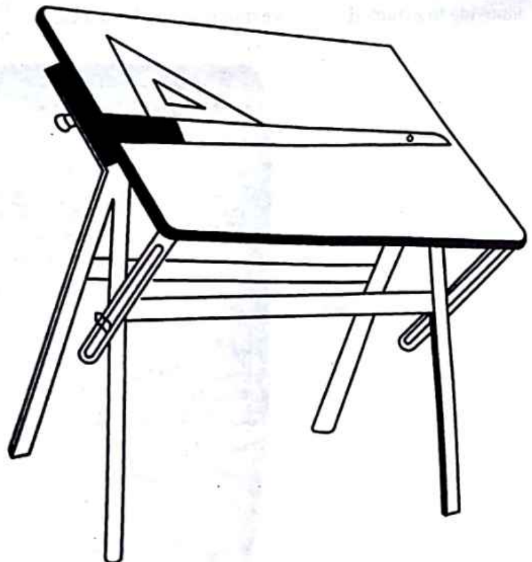
Fig. 1.3 : Trestle for drawing board
