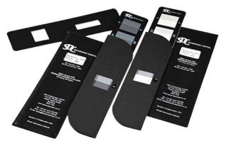
• The grey scale consists of nine pairs of non-glossy neutral grey coloured chips, which illustrate the perceived colour differences. These give a corresponding fastness rating of 5, 4-5, 4, 3-4, 3, 2-3, 2, 1-2, and 1. They are used in the assessment of colour change occurring in fastness tests as described in ISO 105-A02. They are also essential in the grading of light fastness tests when using the Light Fastness Standards.
