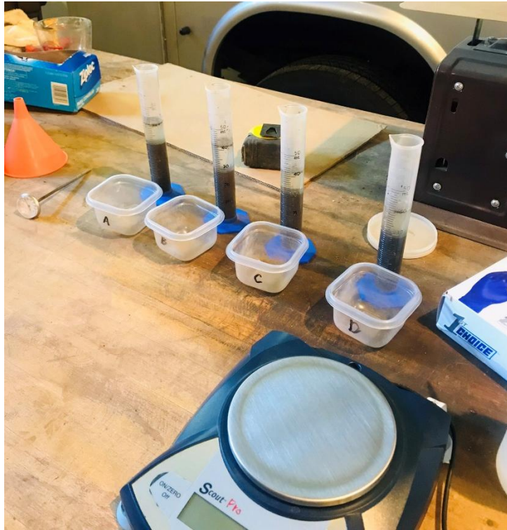
Particle density testing of soil.
