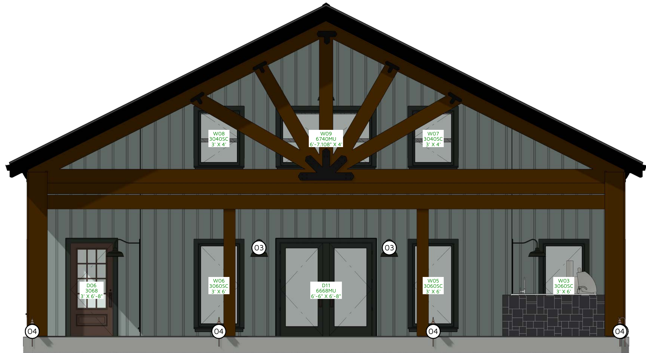
A-4 A-4 EXTERIOR ELEVATION RIGHT 1/4 IN = 1 FT
