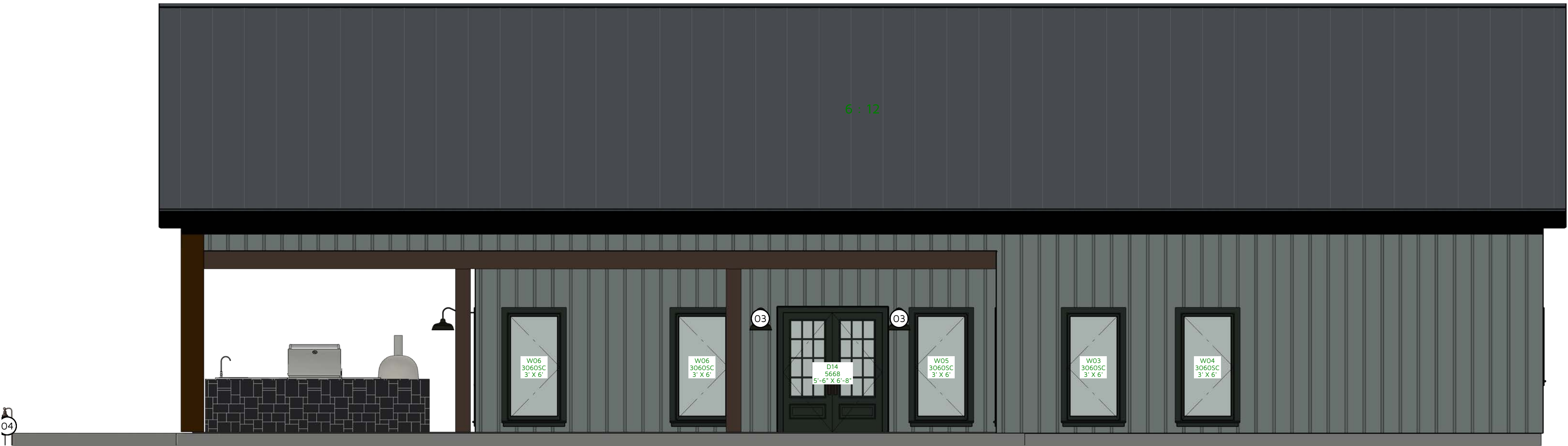
A-2 A-2 EXTERIOR ELEVATION REAR 1/4 IN = 1 FT
