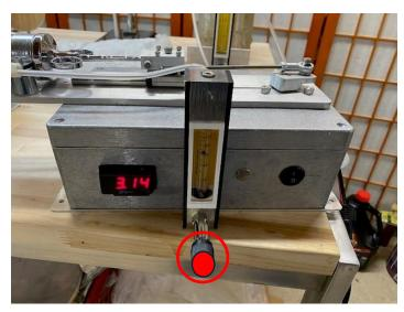
Using the control valve at the bottom of the flowmeter, set the flow to approximately 85 on the black ball scale. If the valve has been adjusted previously, it will retain its adjustment.
