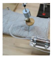
Connect the probe to the breathing machine using 40 cm of tubing with 6 mm inside diameter. The volume of this tube will influence the measurement.
