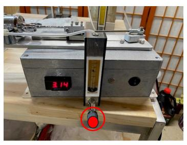
Using the control valve at the bottom of the flowmeter, set the flow to approximately 60 ml/min. If the valve has been adjusted previously, it will retain its adjustment.
