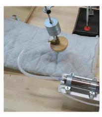
Connect the probe to the breathing machine using 40 cm of tubing with 6 mm inside diameter. The volume of this tube will influence the measurement.
