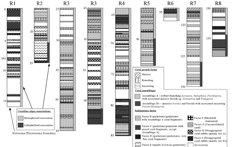
Fig. 4. Individual reef units at Ribbon Reef 5 showing the distribution of coral assemblages, coralline algal associations (data after Braga and Aguirre, 1997) and major sedimentary facies.
