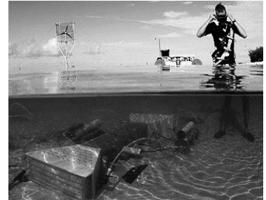
Figure 1: One of the three cpFOCE flumes underwater, with the wind-power generator and floating computer control system in the background. Image © David Kline [3]
