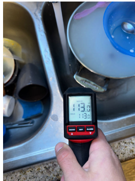
Water temperature noted at 113° F
