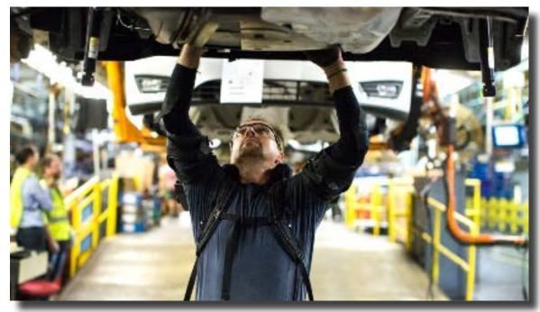
ExoVest is a wearable technology that elevates and supports a worker's arms while performing overhead tasks.
